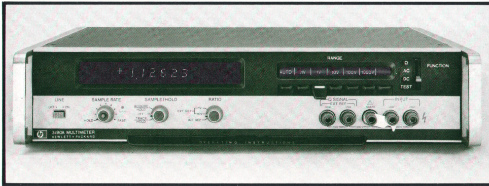
Fig. 1. Model 3490A Digital Multimeter measures dc volts, ac volts and resistance with 10 ppm resolution. Model shown here has Ratio and Sample-and-Hold functions installed. Easy-to-decipher range and function control brings into view only those ranges needed for function selected. Depressing appropriate tab selects range desired. Slide-out instruction card includes operator instructions for using Multimeter to test itself.
